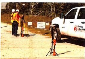
four hours. The collected data showed the gas line depths to be 16.1±0.9 and 15.4±0.8 feet deep. A QL-A Test Hole was excavated where each Duel Spar reading was taken and showed the line depths to be 16.8 and 15.8 feet deep (9 inches and 5 inches difference, and within the confidence intervals reported by the software).
